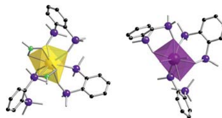
Figure 3. Views of the tricapped trigonal prism ( \text{PuO}_9 ) and square antiprism ( \text{ThO}_8 ) coordination environment.
